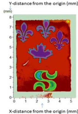
**Fig. 3.** Photoluminescence map of a multi-bandgap GaInAsP/InP QW wafer achieved by irradiation with an ArF laser projecting different masks (2.5X demagnification). The as-grown material emits at 1534 nm. The 'fleur-de-lys' and 'maple leaf' sites emit at 1409 nm and the 'S' site at 1470 nm [15].
