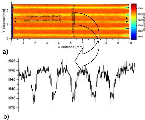
**Fig. 1.** Photoluminescence map of a series of lines of the QWI material fabricated with the Laser-QWI technique (a) and a cross-section PL scan indicating amplitude of the QWI process (b) [12].
