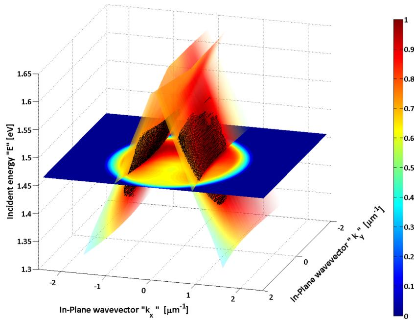
Figure 2 Measured SPR dispersion in  $I(E, k_x, k_y)$  for an integrated QW-SPR architecture. The 3D SPR is extracted from the hyperspectral cube as local maxima, as exemplified by the black dots. The displacement of the 3D SPR in time should provide highly precise spectro-angular information on the biochemical perturbations within the SPs evanescent fields.
