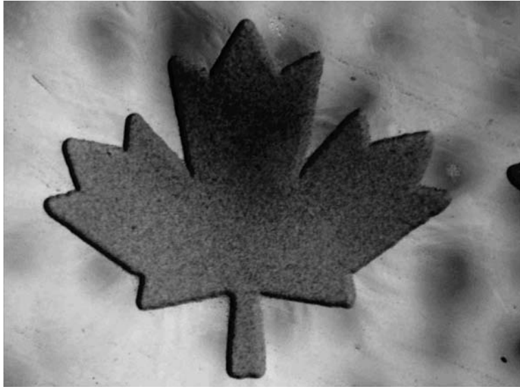
Figure 4.6 A 'Maple leaf' crater etched in Foturan
