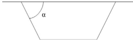
Figure 5.5 Definition of the angle between the original surface and the etched wall ( \alpha )
