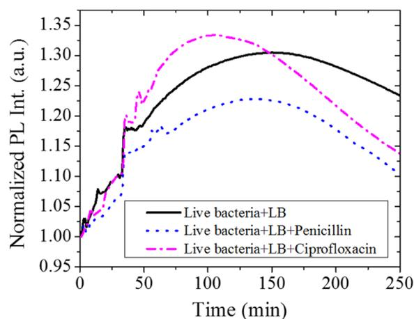
**Fig. 4.** Examples of normalized PL intensity measured in situ for biochips exposed to penicillin resistant, ciprofloxacin sensitive *E. coli* HB101 bacteria and LB (solid line), live *E. coli* HB101 bacteria, LB and penicillin (dotted line), and live *E. coli* HB101 bacteria, LB and ciprofloxacin (dashed-dotted line).
