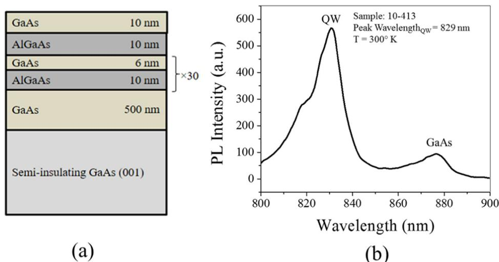
**Fig. 1.** Cross-section of the GaAs/AlGaAs QW microstructure employed for the fabrication of biochips (a), and an example of the PL emission observed at RT from the microstructure irradiated with a 532 nm laser (b).
