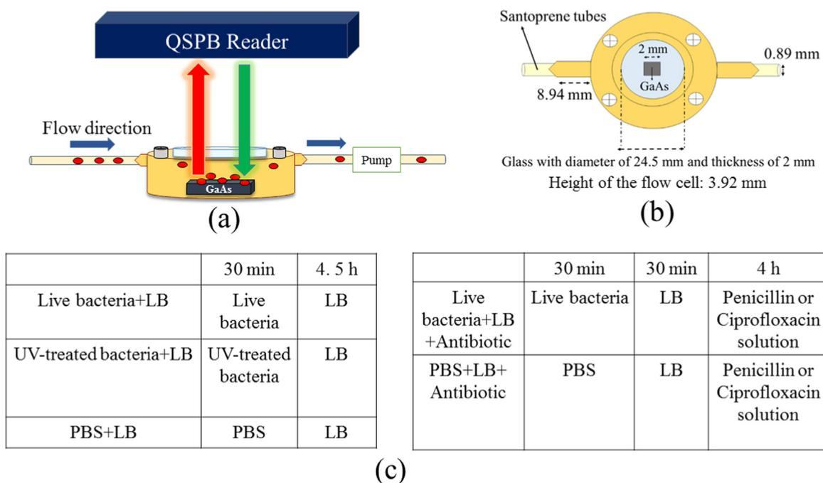
**Fig. 2.** Schematic illustration of the experimental setup (a), top view of the flow cell (b), and time required for different steps of the experiment (c). The biofunctionalized biochips were kept in the flow cell and exposed to bacterial suspension (red ovals) and LB with or without antibiotics while their PL was recorded during the experiment. (For interpretation of the references to color in this figure legend, the reader is referred to the web version of this article.)
