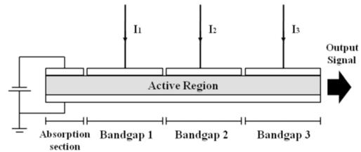
Figure 1. Multi Section SLD profile
