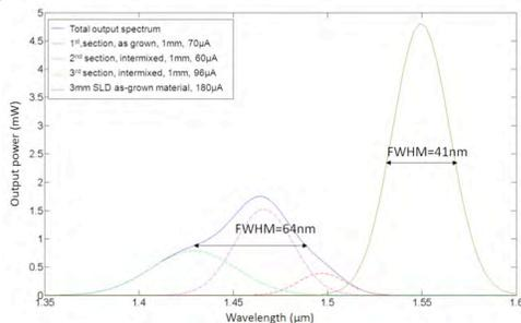
Figure 2. Comparison of two single electrode SLDs, one as grown, one bandgap tuned with 3 different sections of same length
