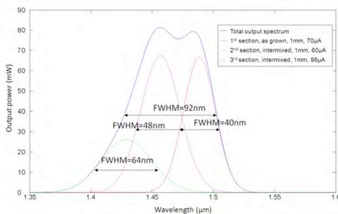
Figure 3. Optimized output spectrum by current tuning
