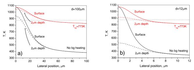
**Fig. 2** Calculated temperature profiles on the surface and 2  $\mu$ m below the surface for a 2-inch InP wafer irradiated by laser beams of 100  $\mu$ m (a) and 12  $\mu$ m (b) diameters. Laser power was adjusted for every simulation to reach the same maximum temperature. Horizontal line indicates the threshold temperature for which a 90-sec RTA induces no significant PL shift [3].
