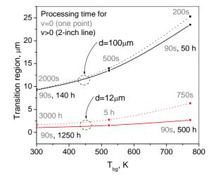
**Fig. 6** Transition widths and processing times to write a 2-inch line of the 100 nm bandgap shifted material at  $T_{max} = 1073$  K. The results at the surface (solid line) and 2  $\mu$ m below the surface (dotted line) have been calculated for 100 and 12  $\mu$ m beam diameters as a function of the background temperature.
