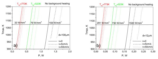
**Fig. 1** Dependence of InP sample surface temperature in the center of the beam  $(T_{max})$  on laser power for different scanning speeds and for beam diameters of 100  $\mu$ m (a) and 12  $\mu$ m (b). Power densities needed to achieve 1073 K with a stationary beam are shown in the picture. Horizontal line – temperature giving 100 nm PL shift in the InGaAs/InGaAsP QW microstructure following the 90-s RTA [3].
