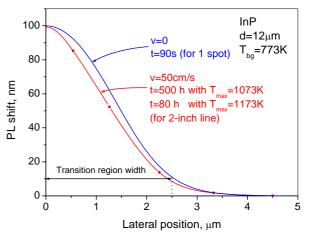
Fig. 4 Calculated intermixing profiles for different scanning speeds.
