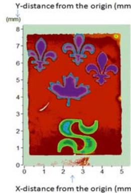
**Fig. 3.** Photoluminescence map of a multi-bandgap GaInAsP/InP QW wafer achieved by irradiation with an ArF laser projecting different masks (2.5X demagnification). The ‘fleur-de-lys’ and ‘maple leaf’ sites emit at 1409 nm and the ‘S’ site at 1470 nm [15].
