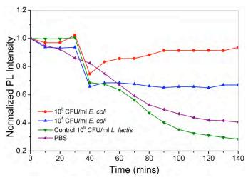
Figure 2. Time-dependent PL intensity signal from an antibody functionalized GaAs/AlGaAs epitaxial microstructure exposed to 10<sup>4</sup> and 10<sup>6</sup> CFU/ml of *E. coli* in a PBS solution. The reference and control experiments were carried out for pure PBS solution and 10<sup>6</sup> CFU/ml of *L. lactis* in PBS.
