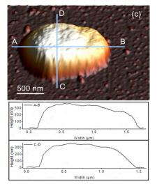
Figure 1. AFM image and cross-sectional scan of an *E. coli* bacterium present on the biofunctionalized surface of GaAs.
