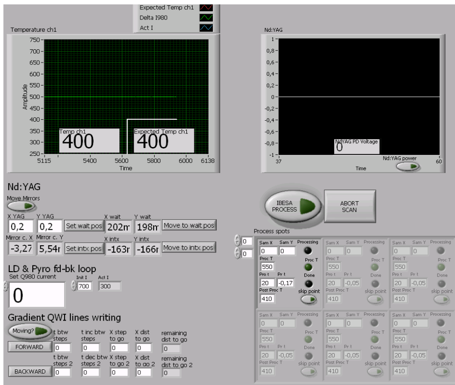
Figure 0.10 LabVIEW based IR Laser – RTA IBESA interface. Automated processing routines.
